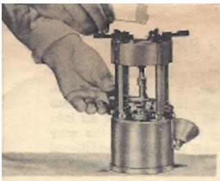
Third — After flame burns steady for 2 or 3 minutes, open Fuel Control Valve AS FAR AS POSSIBLE.
