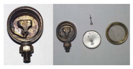
The beginning and end of the hollow spring are soldered.
