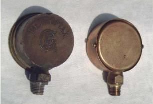
The picture shows two versions, the third one is like the one on the left but has a copper cover to the lower part of the scale inside the glass. So it looks like the one on the right but with a full glass front.
