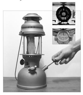
Nose of the grip wheel (#111) has to face upwards. Rocker arm (#223) of the pre heater and ventilating screw (#13) at the manometer have to be closed. Inflate until manometer needle exceeds the red mark.
