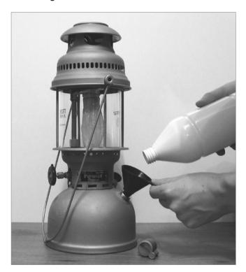
Unscrew manometer (#149). Insert funnel (#65) into the nozzle and pour in pure kerosene (up to 15 mm underneath the nozzle). Readjust manometer tightly. Turn the nose of the grip wheel (#111) upwards.
